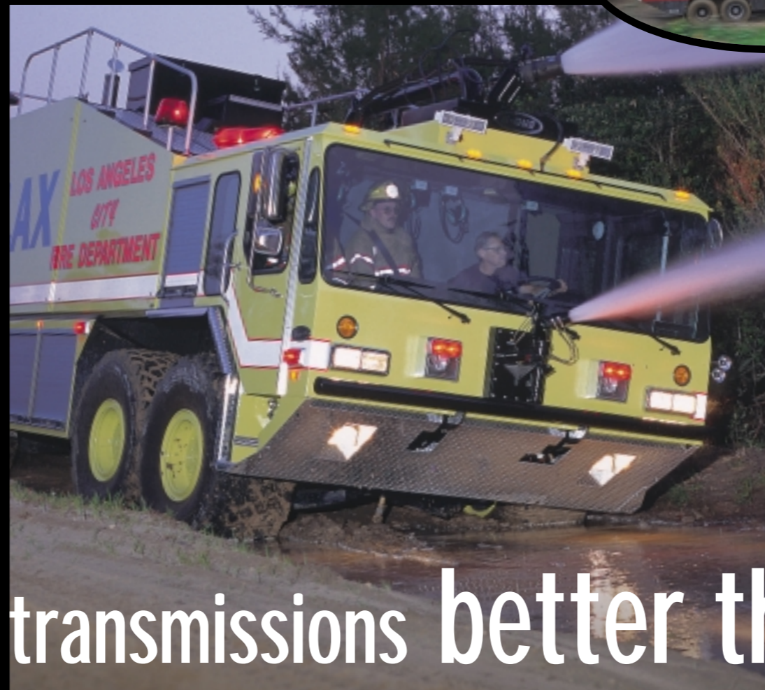
Emergency One's Titan HPR™ 8x8 with its 1000 hp Detroit Diesel engine and Twin Disc TD-61-2619 automatic transmission system can carry up to 4,227 gallons of water and 405 gallons of foam concentrate and still achieve 50 mph in under 30 seconds.
