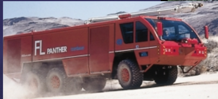
In their Panther series of Aircraft Rescue and Fire Fighting (ARFF) vehicles, Freightliner and Rosenbauer have utilized the latest heavy truck propulsion technologies such as modern 4-cycle, turbocharged diesel engines generating up to 600 horsepower driving through Twin Disc TD61-1180 Six-Speed Automatic Powershift Transmission and Power Divider Systems.
