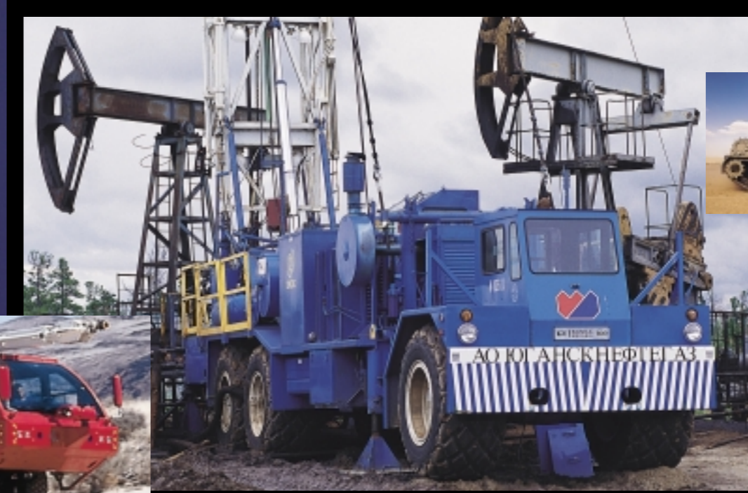
The Twin Disc Transmission System on this highly mobile IRI International oil well servicing rig controls power to the drive axles and well servicing equipment.
