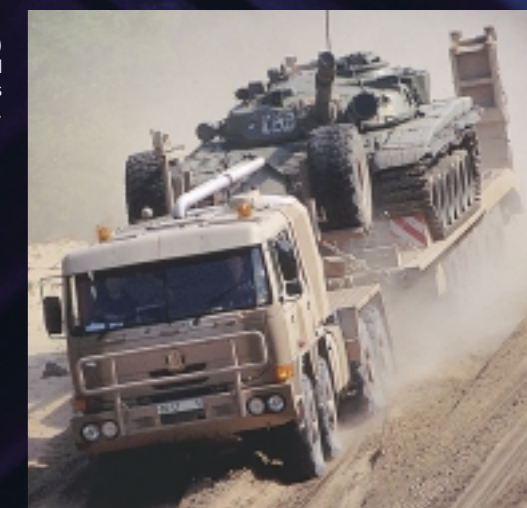
A Tatra HET (Heavy Equipment Transport) equipped with TD-101-3600 10-Speed Automatic Transmission System performs in rigorous desert conditions.
